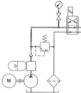
Fig 1.3n Damping pulsations caused by the volumetric pumps.
