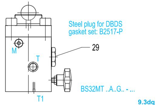
Steel plug for DBDS gasket set: B2517-P
