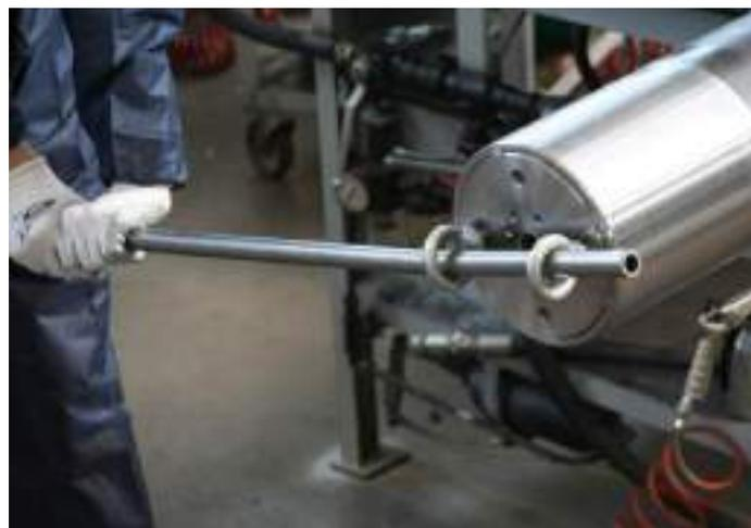
Gas pressure should always be discharged before the disassembly of an accumulator AP. Those accumulators have the oil and gas end caps threaded into the pipe. Always remove the gas cap first – identifiable by the gas valve or by a gas bottle connection.
