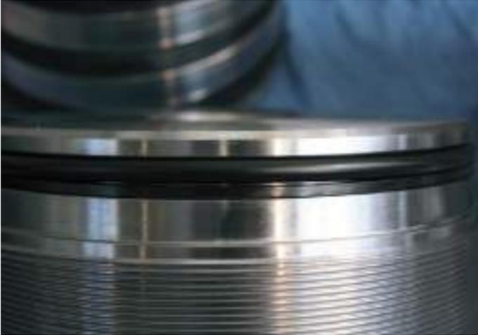
The O-ring and parbak ring, fitted to the accumulator end caps, have a flat face and a concave face to allow the ring and the parbak ring seaying correctly.
