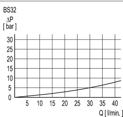
Curves measured using mineral oil with viscosity of 36 cSt at 50°C
