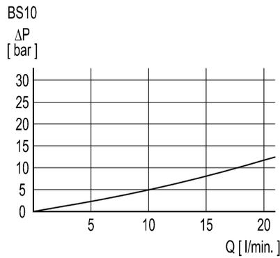
Flow rate from the accumulator via the solenoid valve to the tank
