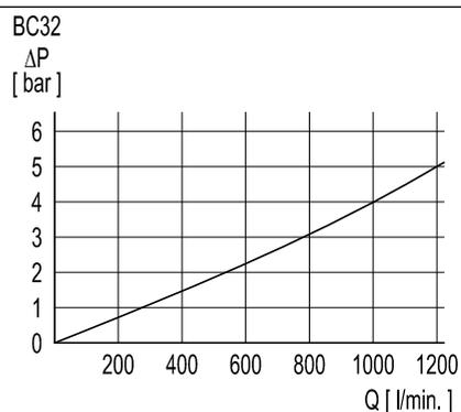
Flow rate from to A and B close to VR
