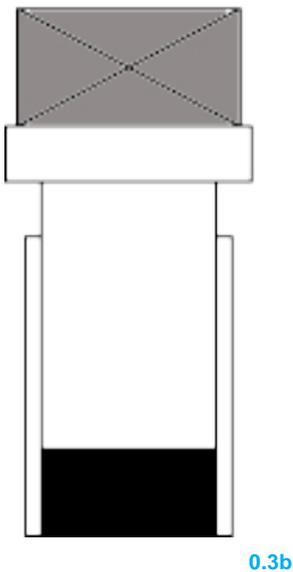
The raised weight Accumulator essentially consists in a vertical steel cylinder inside of which flowed a metal piston on which is placed a weight. The water is pumped into the cylinder so as to raise the piston and the weight; a check valve furthermore prevents the water flowing into the pump. So there is a reservoir of hydraulic energy equal to the product of the cylinder stroke by the weight above.
