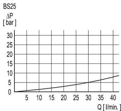
Flow rate from pressure relief valve to tank (only DBDS10)
