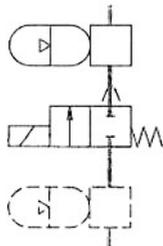
Fig. 1.3o: dampening the pulsations downwards the pump
