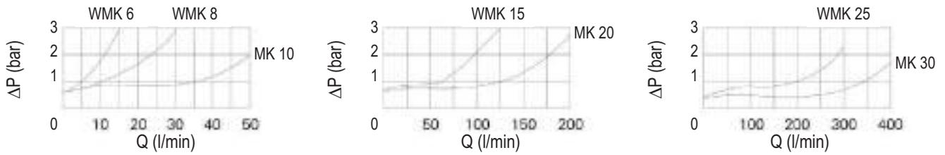
Flow rate via closed check valve with open throttle (measured with viscosity of 36 cSt at 50 °C).
